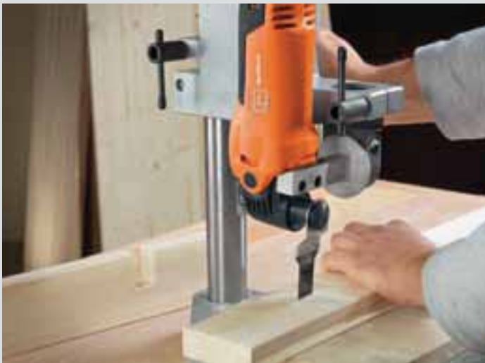
A standard drill jig and the FEIN table and drill jig holder turn the FEIN MULTIMASTER into a stationary machine tool for universal use in the workshop or out on site.
